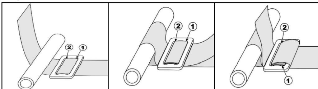
The figure above is the preferred method for harness attachment to harness bar.
